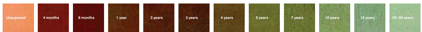
Oxidisation of unwaxed natural copper. Chart used with permission from the Copper Development Association.
