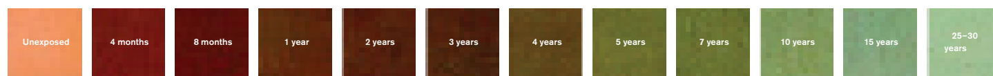
Oxidisation of unwaxed natural copper. Chart used with permission from the Copper Development Association.
